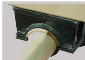
Replaceable nylon bearings on wheel mounts
